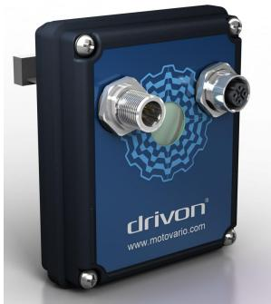
This optional module enables the communication through standard Profibus DPV1 field bus. This module makes it possible to assign a network address through on-board manual rotary selector switches. In addition, the user can activate a termination resistor through jumpers as required. Two M12 B-code connectors (a male and female connector) are provided on the outside of the module for Line connection to field network.
