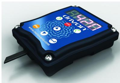
Thanks to the optional keypad and the parameter copy function, the use of Drivon is more practical and quick during the product set-up phase. This function enables to apply the same parameters to inverter motors with the same configuration. In addition it is possible to start the inverter motor in two directions and display several details on the keypad.
