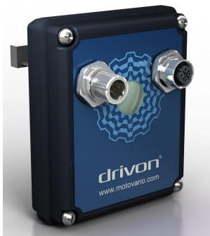
This optional module implements hardware and software interfaces for Real-Time-Ethernet networks over Ethercat profile. Two M12 D-code connectors (a male and a female connector) are provided on the outside of the module for Line connection to field network.
